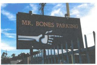
Mr. Bones Logo & Parking Direction 4' H x 8' Plywood Signs Bolted to 4" Steel Box Tubing & 6"D Wood Pole
